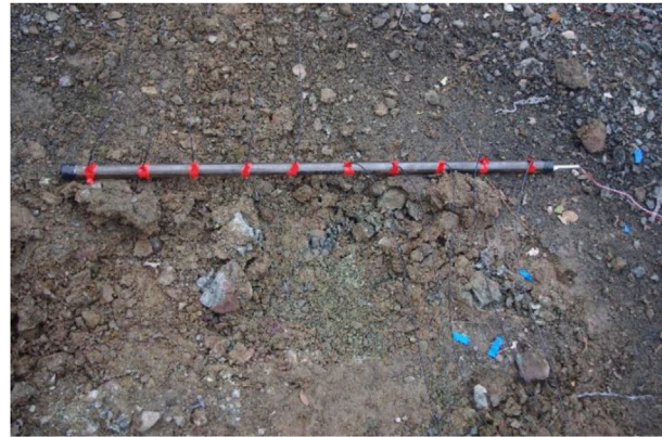
Fig. 3. The steel-charge detonation velocity measurement setup.
