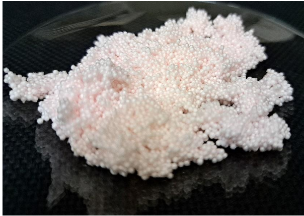
Figure 3. Low-density emulsion matrix based mixture
