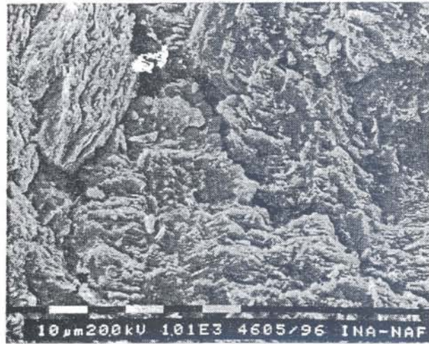
Fig. 3. Scanning electron micrographs of tested samples: a – microfractures in diabase sample Brensbreg are sparse and microblocks are formed only sporadically, b – microfractures in diabase sample Žervanjska 1 are very sparse and isolated, so microblocks are not formed, c – microfractures in diabase sample Žervanjska 2 are sparse and isolated, so microblocks are not formed, d – microfractures in diabase sample Hruškovec are sparse and microblocks are formed only sporadically (Tomašić et al., 1997), e – microfractures in andesite sample Fužinski Benkovac are abundant, clearly visible and intertwined, so numerous microblocks are formed (Tomašić et al., 1997).
