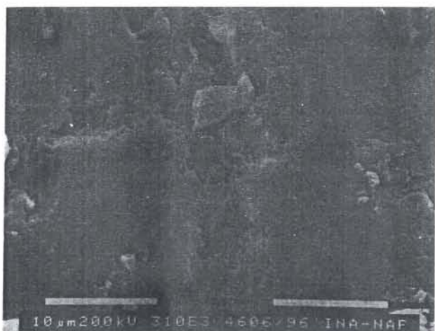
Fig. 7. Surface of dolomite after polishing (bar = 10 μm). Strongly outlined »vuggy« porosity. Crystals of dolomite show a skeletal rim.
