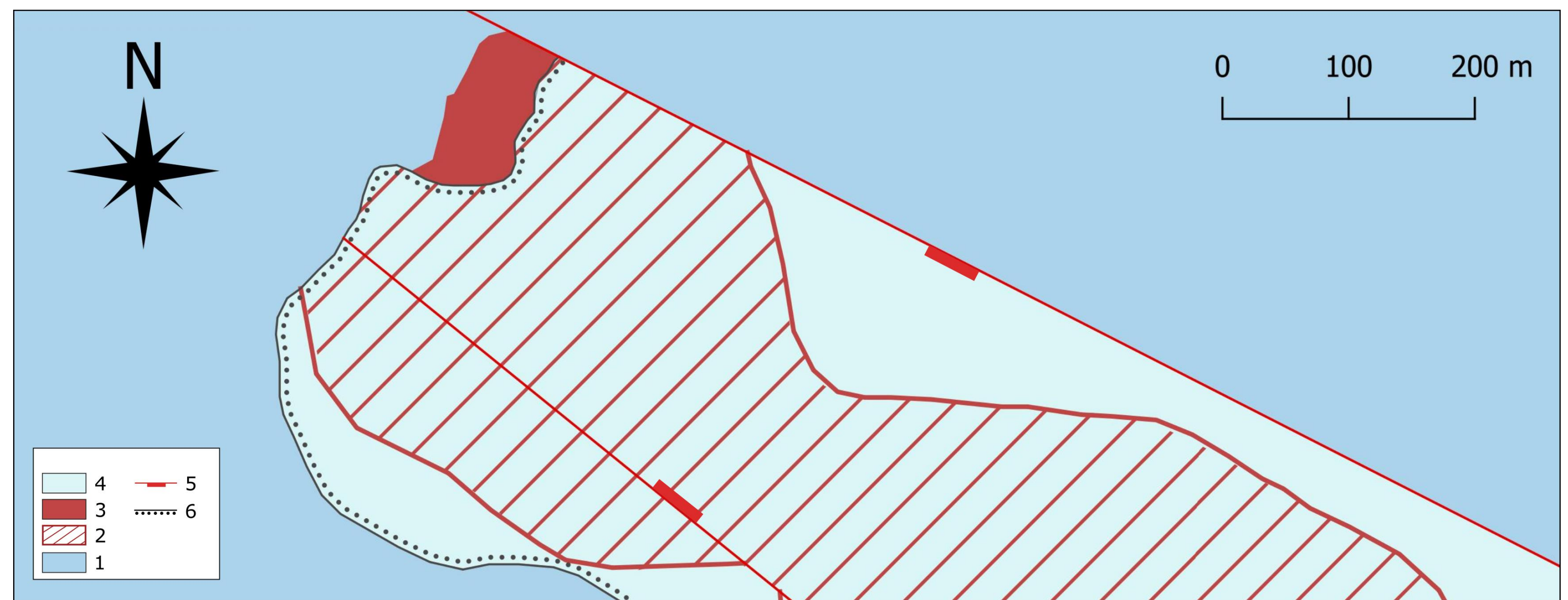
Figure 2. Geological map of the Rovinj-1 deposit, based on the data provided by the GEO-5 company, 1 – Muča unit, 2 – extent of the bauxite body below the Kirmenjak unit, 3 – bauxite, 4 – Kirmenjak unit, 5 – normal faults, 6 – unconformity.
