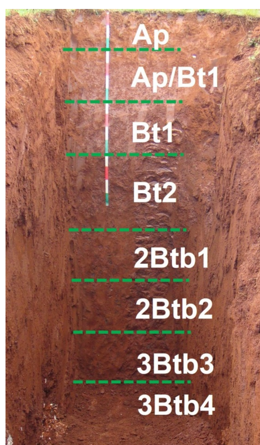
Figures 2 and 3: The studied profile (left) and the PPL microphotograph of the Bt2 horizon at the boundary with the 2Btb1 horizon (right) - blocky microstructure with accommodated and partially accommodated subangular peds is well developed; partially relict, dusty clay coatings/infillings are observable along the plane void that forms the abrupt boundary between the Bt2 and 2Btb1 horizons.
