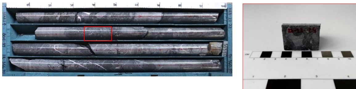
Figure 5-6. The position of the sample MOB-BRD-27-22-24 is framed by the red rectangle (left figure obtained from Adriatic Metals Ptc.).
