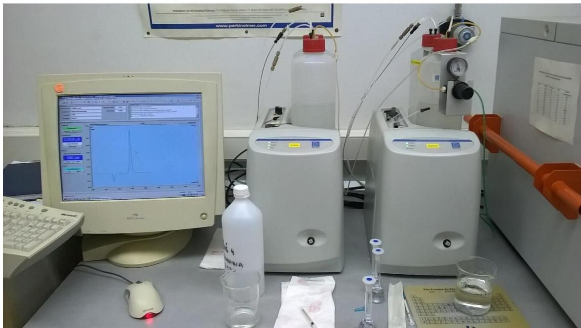
Slika 3 - 4 Ionski kromatograf (ICS-1000 Ion Chromatography System, Dionex)
