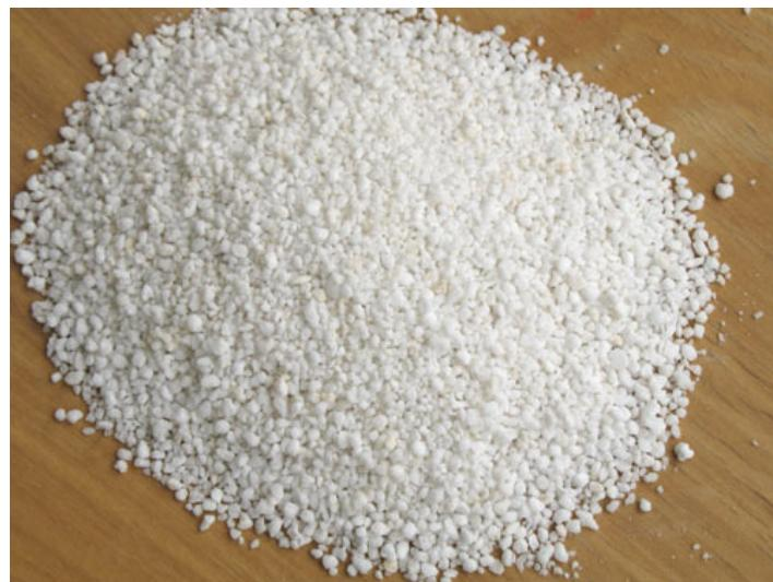
**Slika 4-1.** Zrnca perlita (<http://www.renova.com.mk/en/perlit.html>).
