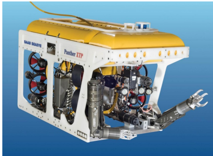
Slika 2-3. Daljinski upravljana jedinica (engl. Remotely Operated Vehicle – ROV ) ( www.offshoreenergytoday.com )
