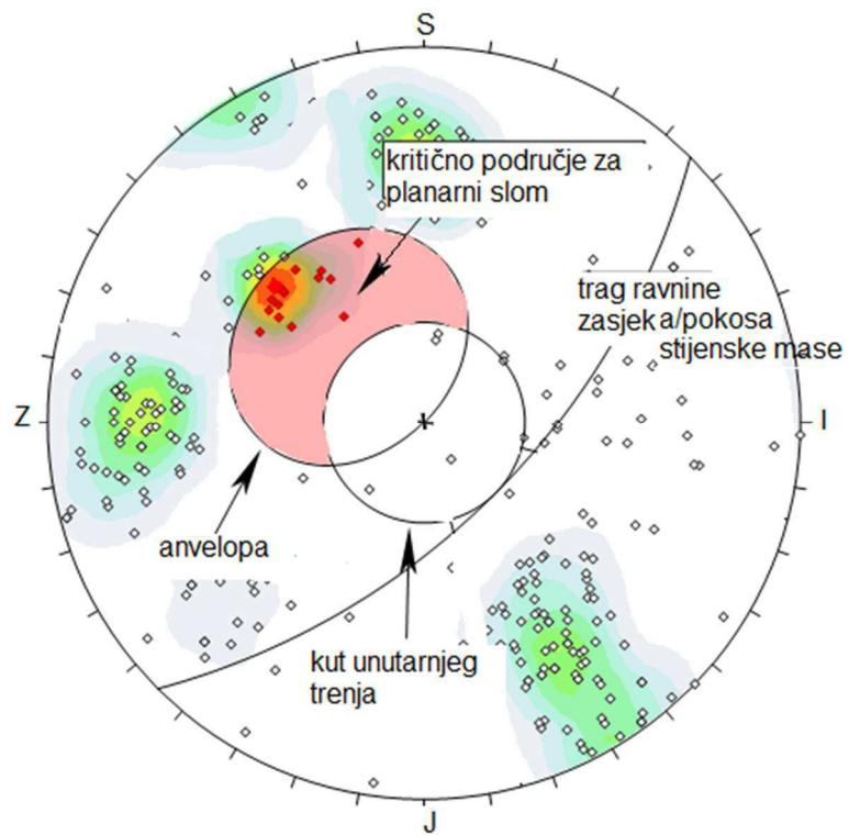
Slika 3.8. Stereografska projekcija za planarni slom (modificirano prema [https://www.rockscience.com/help/dips/webhelp/dips/Planar\\_Sliding.htm](https://www.rockscience.com/help/dips/webhelp/dips/Planar_Sliding.htm))
