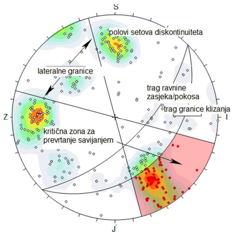
Slika 3.13. Stereografska projekcija za prevrtanje savijanjem (modificirano prema [https://www.rocscience.com/help/dips/webhelp/dips/Flexural\\_Toppling.htm](https://www.rocscience.com/help/dips/webhelp/dips/Flexural_Toppling.htm))
