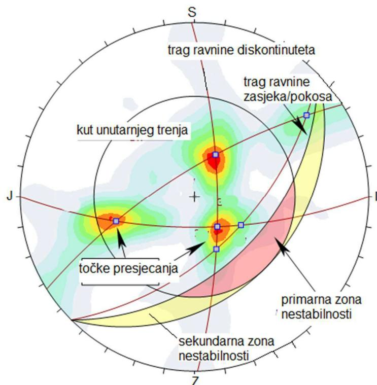
Slika 3.10. Stereografska projekcija za klinasti slom (modificirano prema [https://www.rockscience.com/help/dips/webhelp/dips/Wedge\\_Sliding.htm](https://www.rockscience.com/help/dips/webhelp/dips/Wedge_Sliding.htm))
