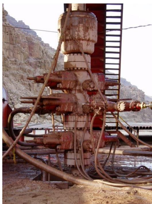
**Slika 7-1.** Preventerski sklop (<http://www.iwcfdrillengineer.com>)
