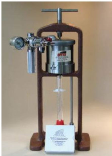
Slika 5-10. API filter preša (OFI Testing Equipment, 2018 (e))
