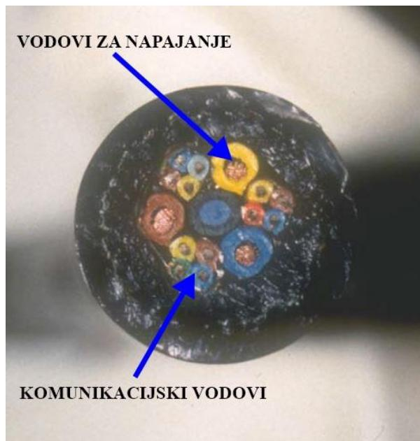
Slika 3-6. MUX kabel (Imperial Oil And Exxonmobile, 2009)
