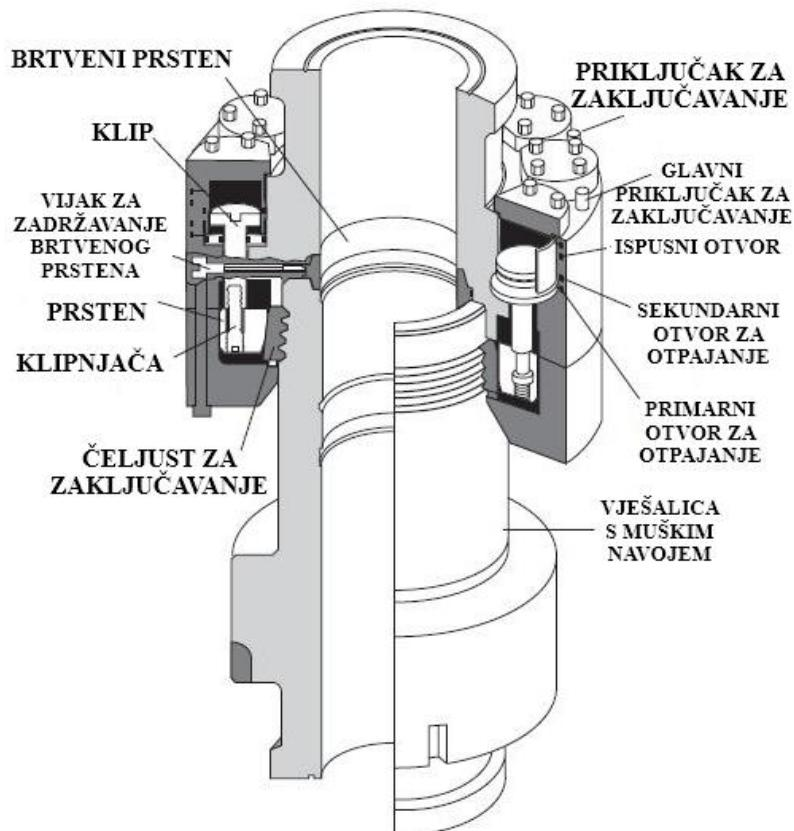
Slika 2-22. Dijelovi hidrauličke spojnice (Aberdeen Drilling School, 2002)
