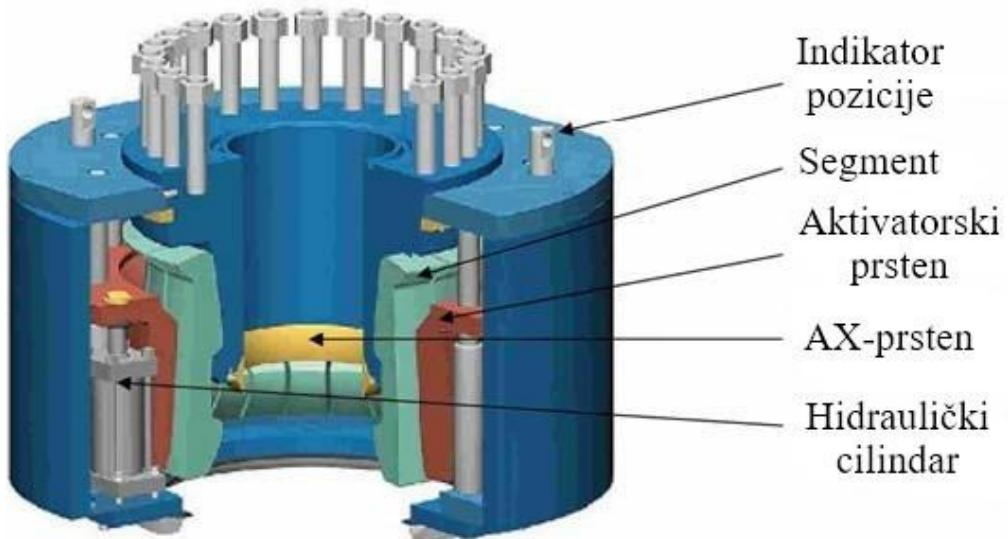
Slika 2-21. Hidraulička spojnica (Jaap Peetsold)
