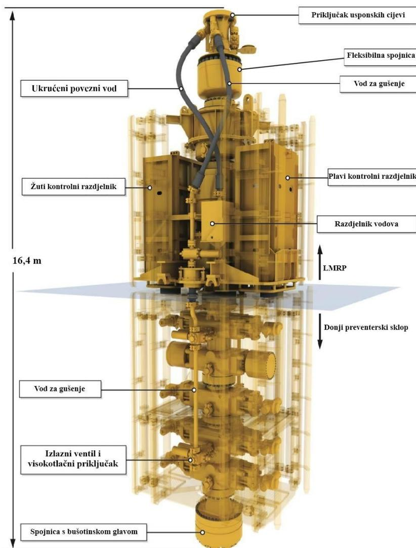
Slika 2-1. Podvodni preventerski sklop platforme Deepwater Horizon (Transocean, 2011)
