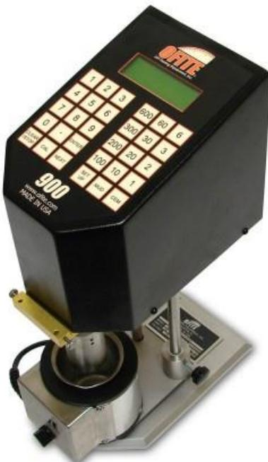
**Slika 5-1.** Model korištenog viskozimetra (OFI Testing Equipment Inc., 2015)
