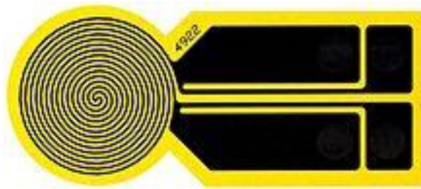
Slika 4-3: TPS senzor, model Hot Disk 4922, radijus spirale oko 15 mm. Preuzeto s http://en.m.wikipedia.org/wiki/Thermal_conductivity_measurement
