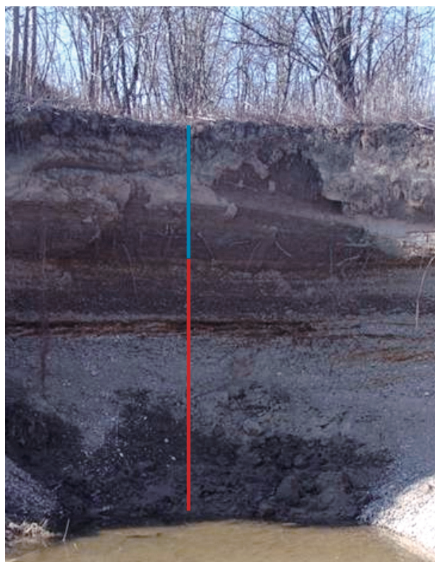
Figure 4. Unsaturated zone profile. Legend: Blue label – soil (approx. 2 m); red label – gravels and sands (approx. 3.5 m)
