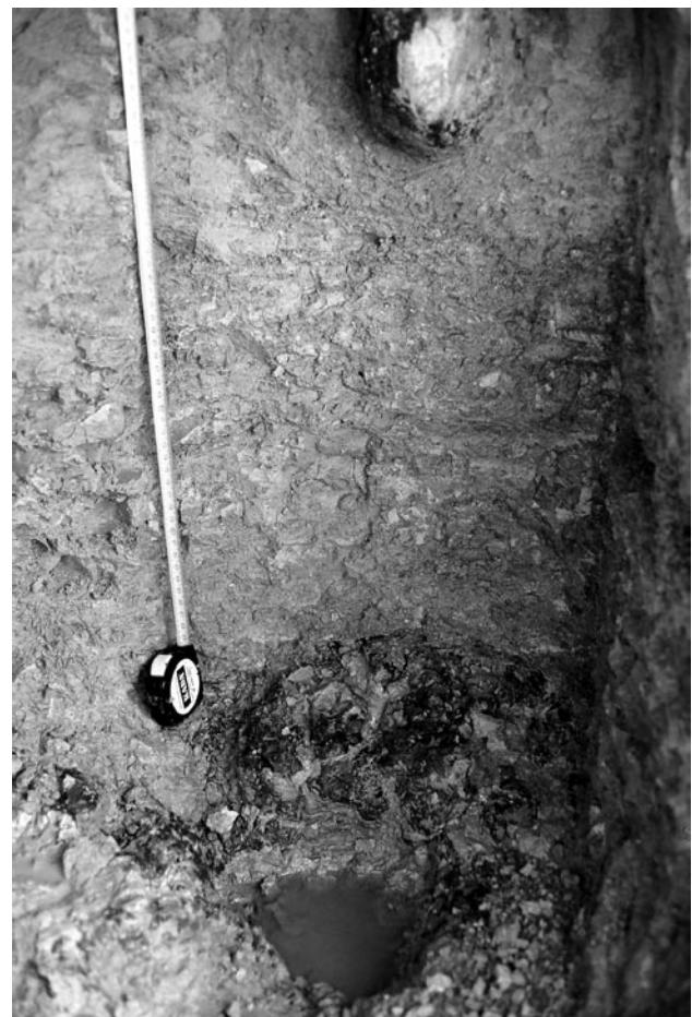
Fig. 22 Contact between greenish-grey clays and karstified "Istarski žuti" limestone (Tri jezerca quarry).
