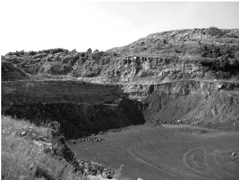
Fig. 7 Bauxite deposit Rovinj–1. Contact of bauxite and first part of the second transgressive–regressive large-scale sequence of Jurassic–Cretaceous shallow-water carbonates.
