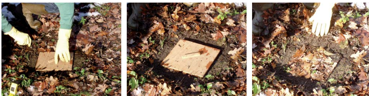
Figure 4. Sampling of organic layer on the soil surface
