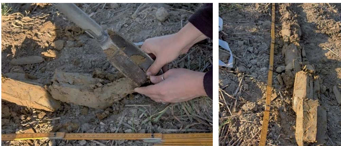
Figure 3. and 4. Soil sampling by probe
