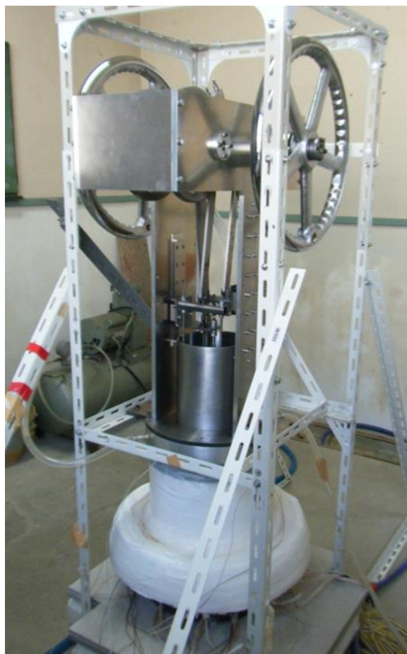
Slika 3-7. Nisko temperaturni model snage 250 W, Japan (Isshiki, 2012)
