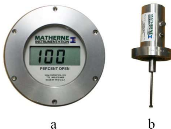
Slika 2-20. Indikator i senzor pomaka podesive sapnice (Matherne Instrumentation, 2020 e)
