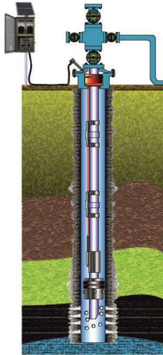
Slika 5- 3. Proizvodni niz opremljen permanentnim dubinskim manometrom ( https://docs.google.com/viewer?a=v&pid=sites&srcid=bm92YXRlY2hydXMuY29tfHd3dy1ub3ZhdGVjaHJ1cy1jb218Z3g6NmEwNjZkMGI2YjA5NTgxYQ )
