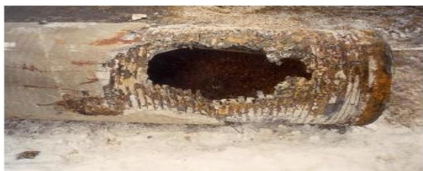
**Slika 3-5.** Korozije cjevovoda u tlu (<https://corrosion-doctors.org/SoilCorrosion/>, 14.08.2020.).
