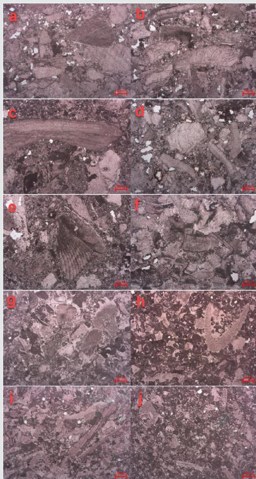
**Figure 6:** Microphotographs of limestone samples: a) Su2 – packstone/biomicrite; b) Su1 – packstone/ biomicrite; c) Su3 – packstone-to-floatstone/biomicriteto-biomicrudite; d) Su4 – packstone-to-floatstone/ biomicrite-to-biomicrudite; e) Su5 – floatstone/ biomicrudite; f) Su8 – packstone/ biomicrite; g) Su9 – packstone/biomicrite; h) Su7 – packstone/biomicrite i) Su11 – packstone/biomicrite; j) Su12 – packstone/ biomicrite.
