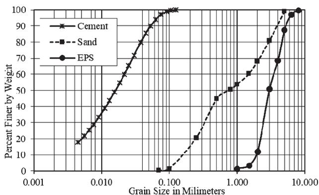
Figure 1: Granulometric composition of cement, sand and EPS
