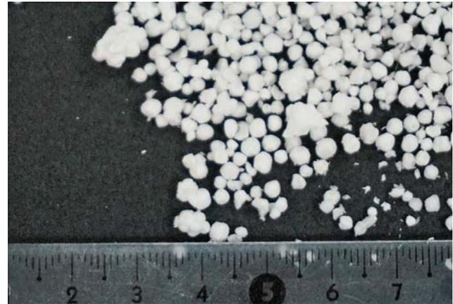
Figure 2: Granulated waste EPS
