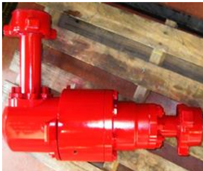
Slika 3-14. Rotirajuća spojnica (Rui tai mechanical & electrical, 2013)
