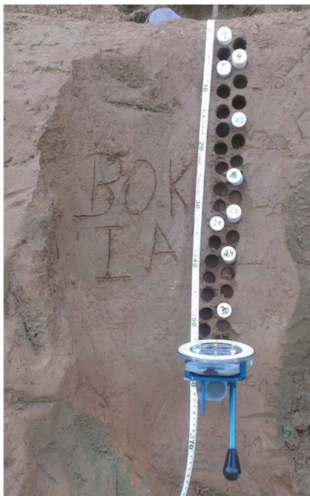
Izuzimanje uzoraka za paleomagnetna mjerenja (Bok, otok Susak) / Sampling for palaeomagnetic measurements (Bok section, Island of Susak)
