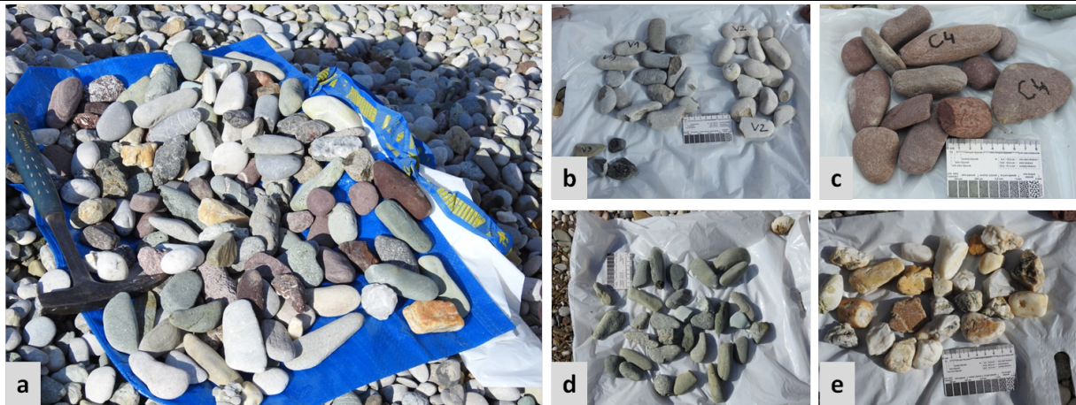
Figure 3: Bulk sample of gravels (a) and clast sorted into categories: (b) – carbonates; (c) – red sandstones; (d) – green sandstones; (e) – quartz(ites) and cherts. Collected in gravel pit "Abesinija" in March 2020.
