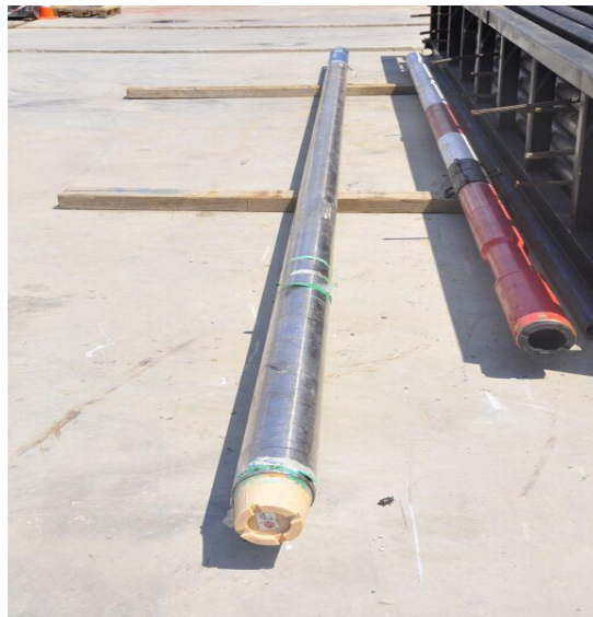
Figure 5-3. Non – magnetic drill collar (Aydin, 2015)
