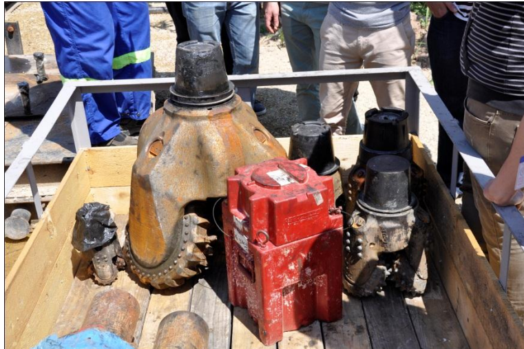
Figure 8-1. A typical large diameter bit used in geothermal drilling ( Aydin, 2015)
