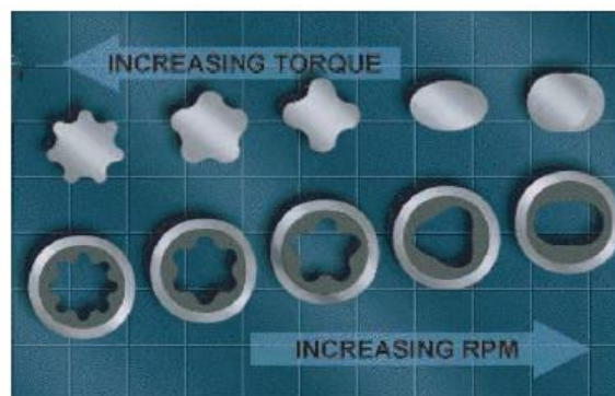
Figure 6-4. Typical rotor / stator configurations (www.BakerHughes.com)
