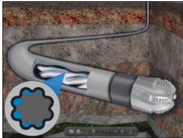
Figure 6-1. Schematic figure of a PDM ( www.laser-ndt.com )
