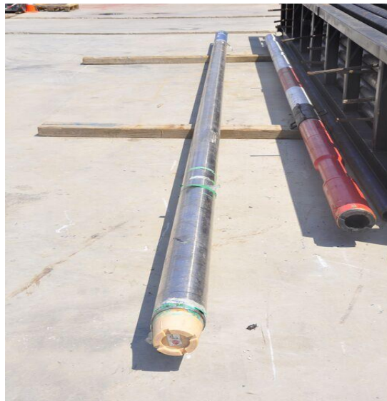
Figure 5-3. Non – magnetic drill collar (Aydin, 2015)
