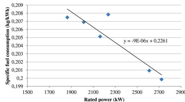
Figure 1 Specific fuel consumption related to engine power
