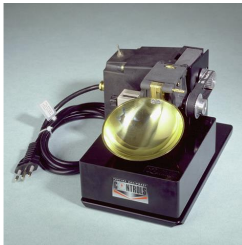
Slika 4-17. Casagrandeov uređaj (preuzeto s https://www.controls-group.com )
