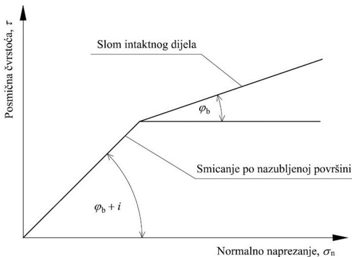
**Slika 2-3.** Pattonov bilinearni model smicanja (Patton, 1966)
