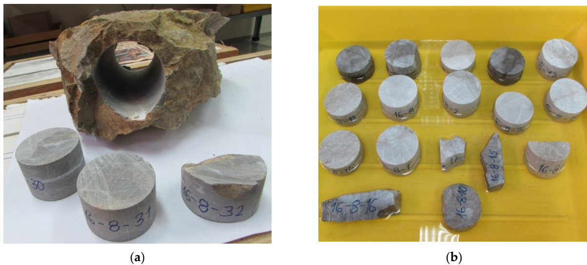
Figure 3. Samples of test material: (a) field samples from which cored samples were made for testing; (b) part of the prepared samples of regular and irregular geometry.
