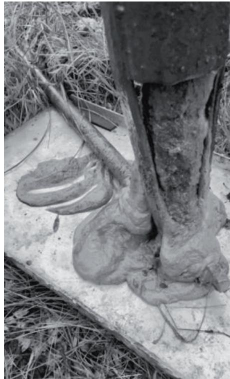
Fig. 9. Liquid gyttja sampled from one of the boreholes (Fot. P. Pietrzykowski)
