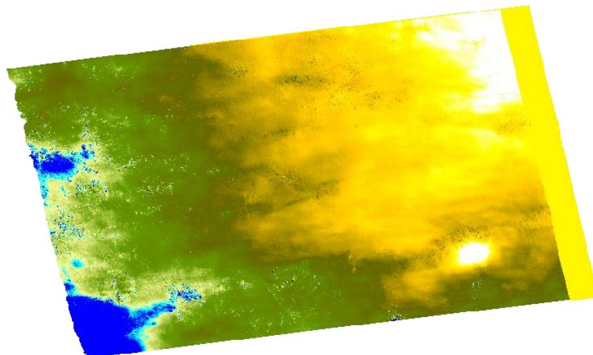
Slika 5.7 Obrada podataka Range Doppler Terain Correction operaterom.
