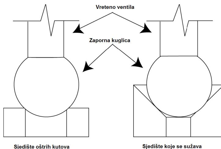
**Slika 3-2.** Konfiguracije sjedišta kuglice ([https://petrowiki.spe.org/Gas\\_lift\\_valve\\_mechanics](https://petrowiki.spe.org/Gas_lift_valve_mechanics))
