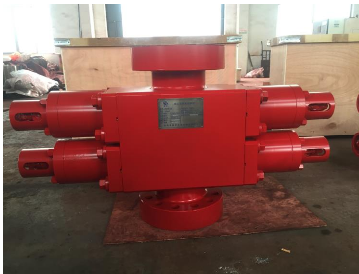
Slika 3-8. Čeljusni preventer ( https://jielin.en.made-in-china.com , 2014)
