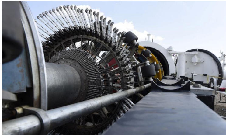
Slika 3-1. Čistači cjevovoda ( https://www.tcenergy.com/stories/ , 2017)
