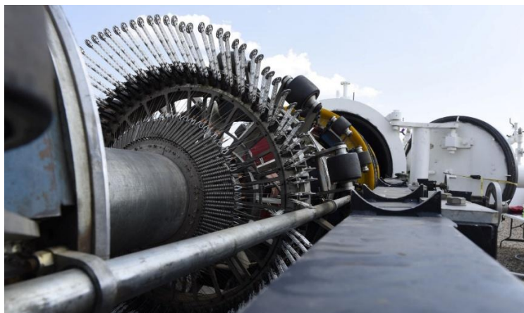
Slika 3-1. Čistači cjevovoda ( https://www.tcenergy.com/stories/ , 2017)
