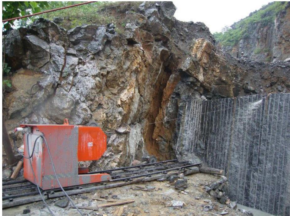
Slika 3-3: Dijamantna žična pila pri radu (<https://www.xmsinostar.com/wp-content/uploads/p2-diamond-wire-saw-machine-for-marble-quarry-cutting.jpg>)
