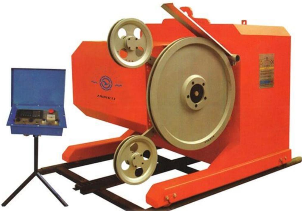
Slika 3-1: Postrojenje dijamantne žične pile (<https://www.xmsinostar.com/wp-content/uploads/Diamond-Wire-saw-machine-for-marble-granite-quarry.jpg>)
