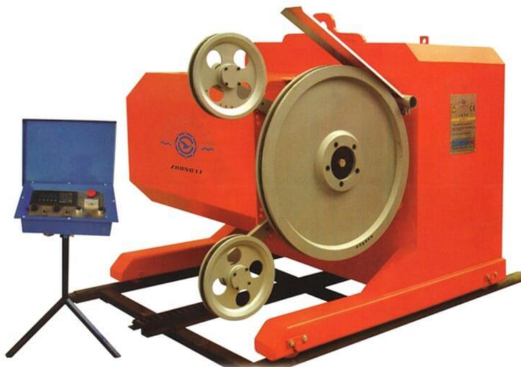
Slika 3-1: Postrojenje dijamantne žične pile ( https://www.xmsinostar.com/wp-content/uploads/Diamond-Wire-saw-machine-for-marble-granite-quarry.jpg )
