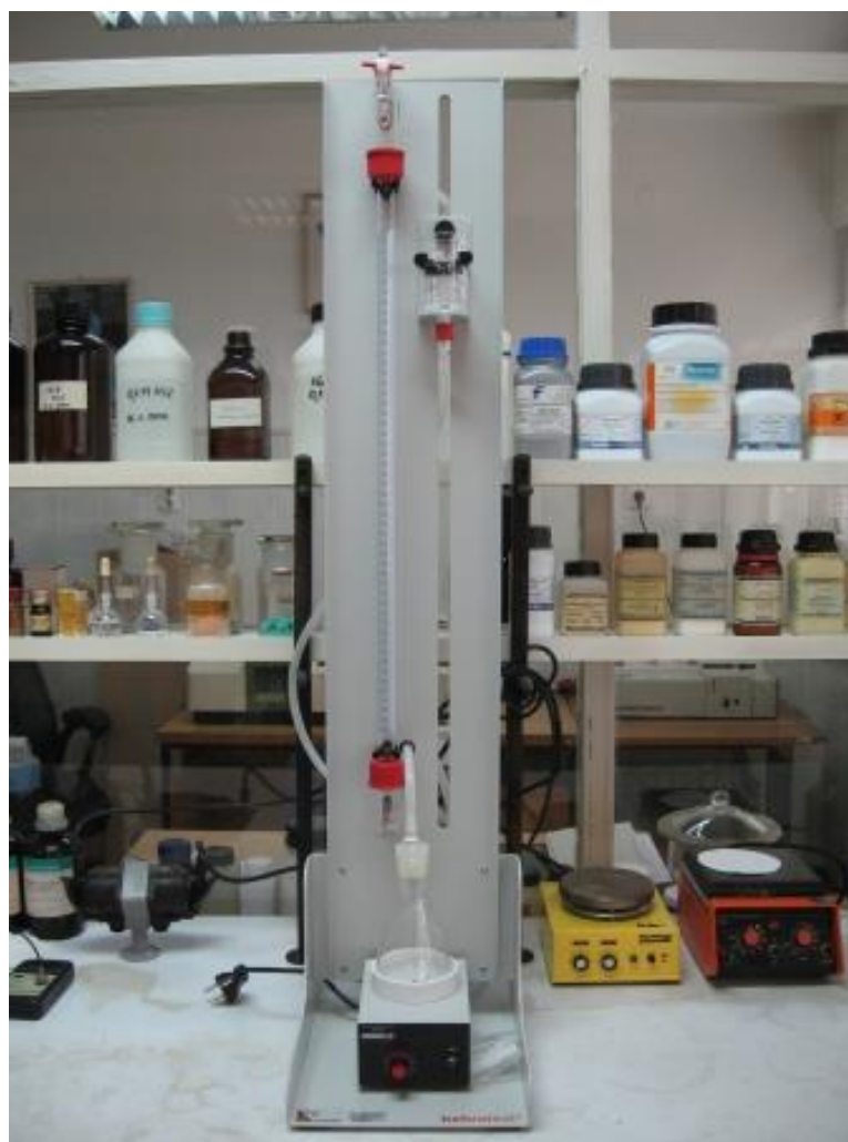
Slika 3.4. Scheibler-ov kacimeter (preuzeto s: https://sestar.irb.hr/instrumenti_show.php?ID=1263 )
