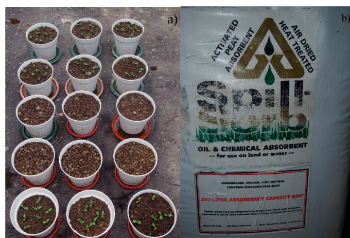
Figure 2. (a) Experimental set up. Picture taken at the end of the study (153 days); (b) bioremediation treatment, Spill-Sorb.
