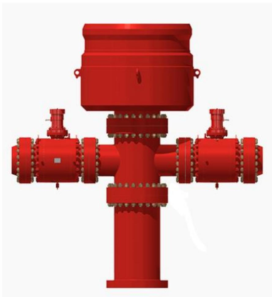
**Slika 7-1.** Prikaz diverterskog sklopa ([www.drillingformulas.com](http://www.drillingformulas.com), 2021)
