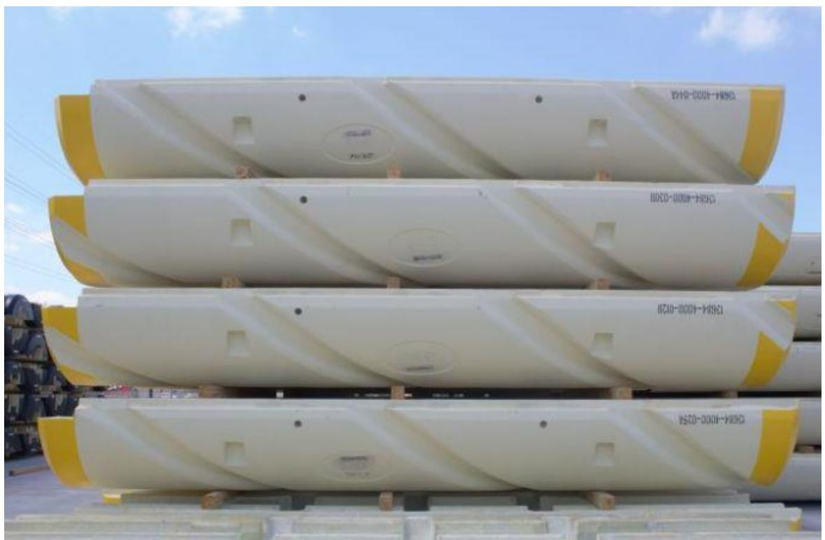
**Slika 3-6.** Uzgonski moduli s helikoidalnim rebrima ([www.crpsubsea.com](http://www.crpsubsea.com), 2022)
