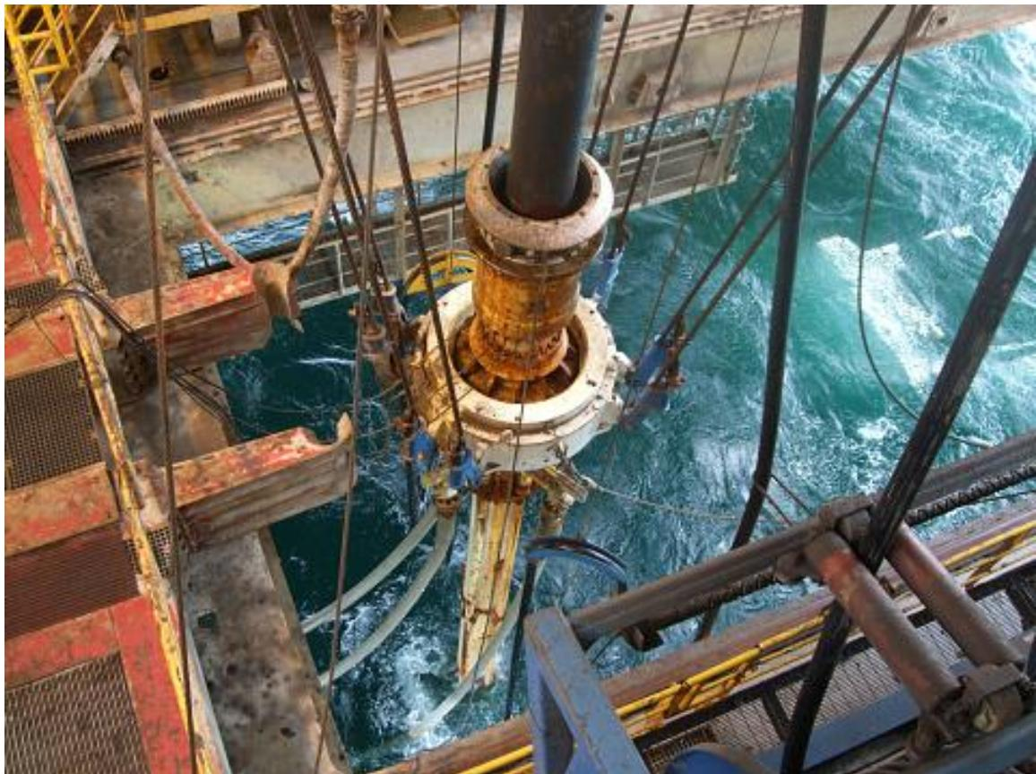
Slika 5-2. Prikaz teleskopske spojnice u radnom okruženju ([www.istockphoto.com](http://www.istockphoto.com), 2011)
