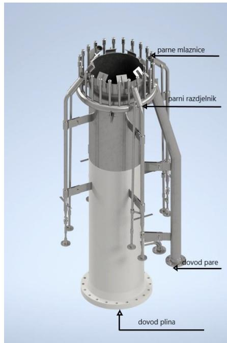
**Slika 4-1.** Baklja s dovodom pare (Encore Combustion, 2022)
