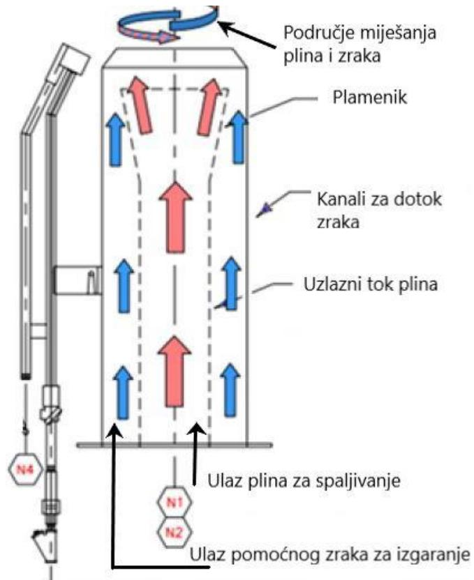
**Slika 4-2.** Baklja s dovodom zraka (Park, 2020)
