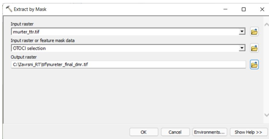
**Slika 4-15.** Izrada *Extract by Mask* otoka Murtera
