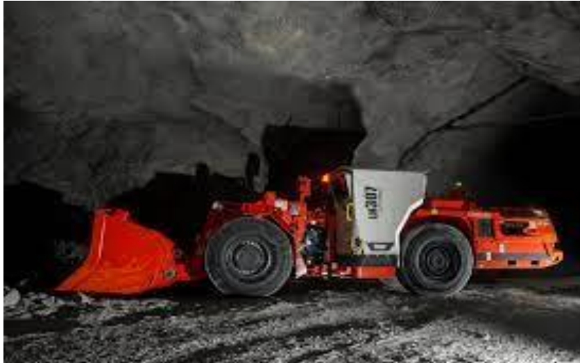
Slika 2-1. Dizelski LHD utovarivač ( Sandvik mining and rock technology )
